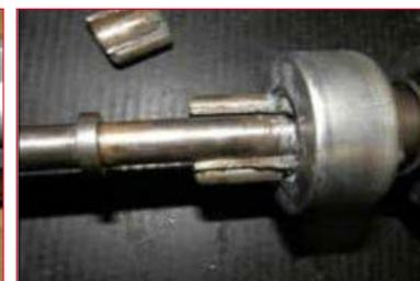
**Side loading** occurs when the starter is not properly installed to the engine block (loose or binding). During the crank cycle, the starter is attempting to turn the engine over. If the housing of the starter is loose or misaligned, the starter drive is forced to walk over the engine flywheel teeth. This violent action creates severe side loading on the starter housing and engine mounting surfaces. This action can cause the starter nose housing or engine block mounting area to fracture.
