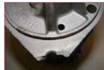
**Starter housing** damage can also occur by over torqueing or uneven torqueing when being installed.
